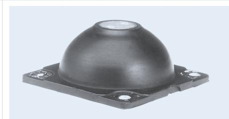
The TT-A mount is a mid frequency isolator which combines a low profile and large deflection capability in order to provide both shock and vibration protection. The TT-A is ideal for applications where high amplitude vibration inputs are expected or where large shock deflections are needed.
